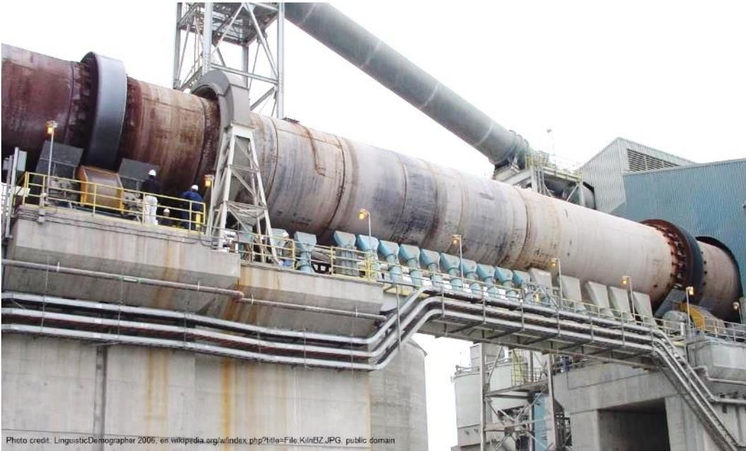
**Figure 20: Kiln in the cement industry, as an example for future application of high-temperature solar process heat**
