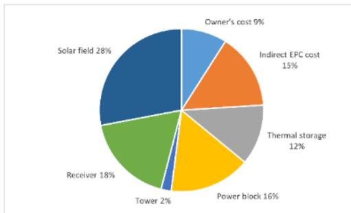
**Figure 59: Cost breakdown of a CSP plant based on solar power technology. Source: [31]**
