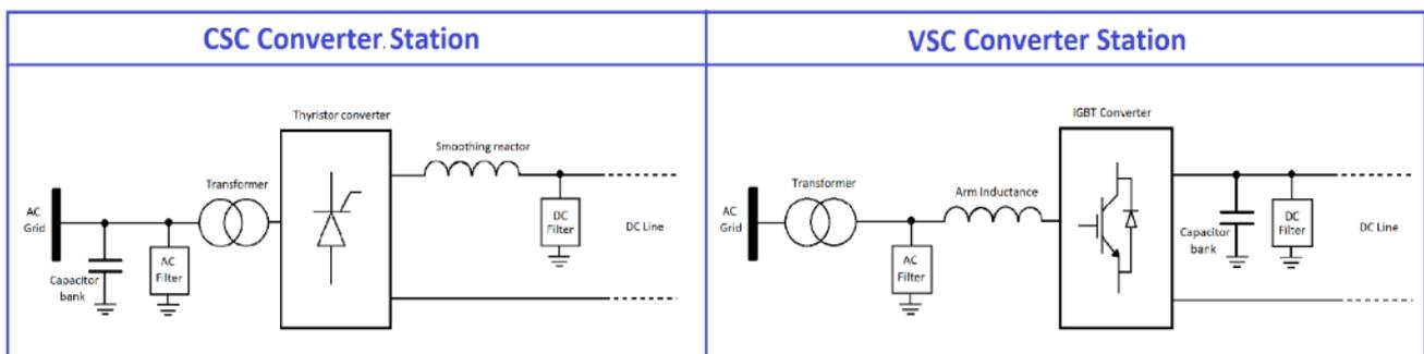
Figure 89. HVDC Technologies: CSC Converter and VSC Converter [197]
