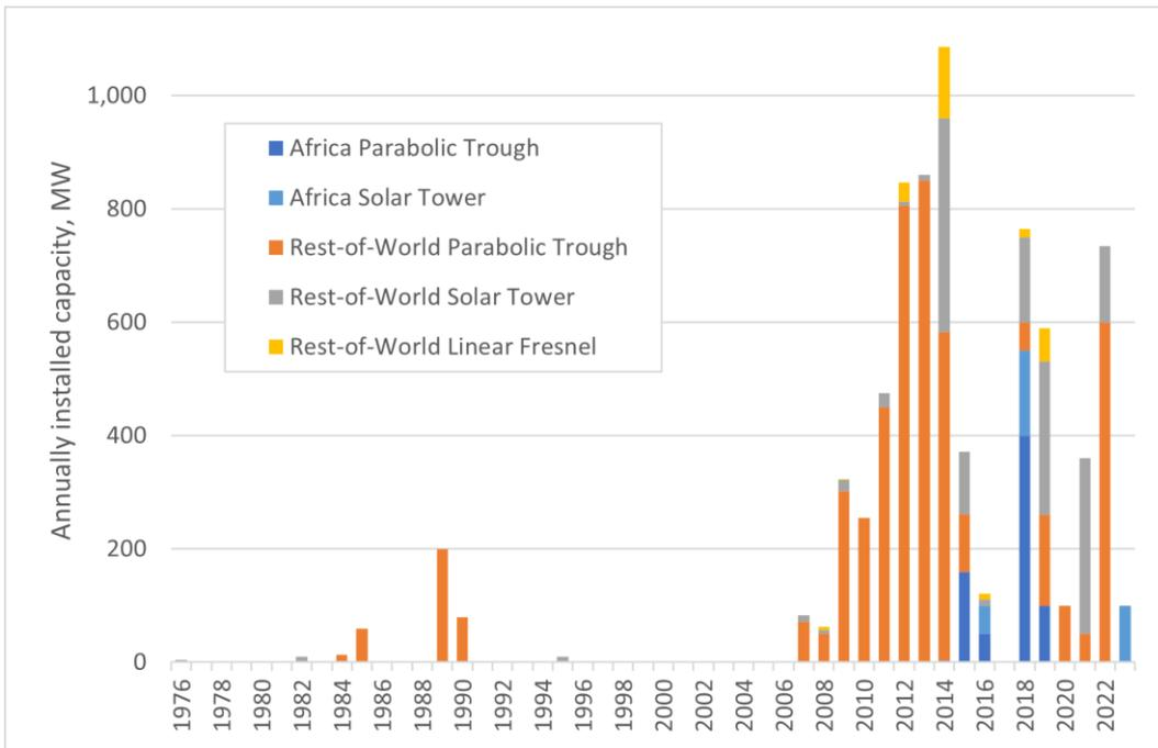
**Figure 13: Annually installed CSP capacity for Africa and Rest-of-World, for three technologies, Parabolic Trough, Solar Tower, and Linear Fresnel concentration modes. Source [2]**
