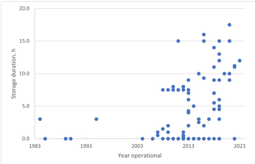
Figure 14: Storage duration in hours at rated capacity, for CSP plants listed in [2]
