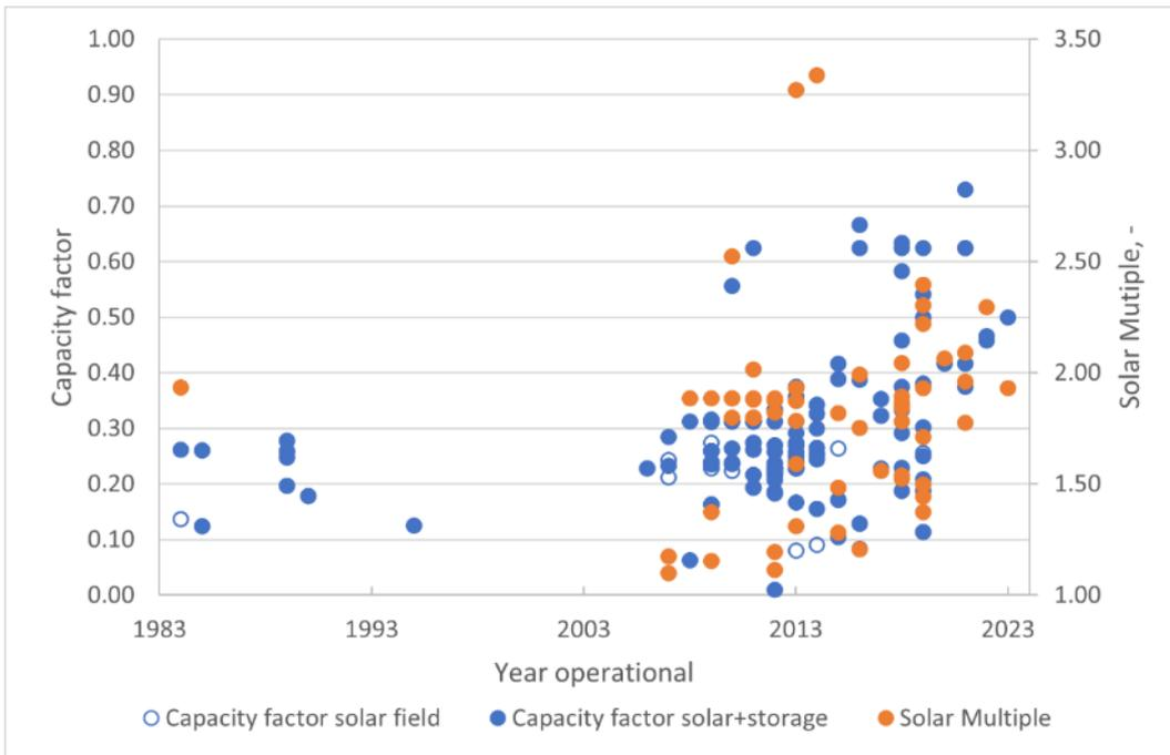
Figure 17: Capacity factors and Solar Multiple of most operational CSP plants (excluded are experimental plants, and plants where data has been found to be incomplete or incoherent). Source [authors] [2]
