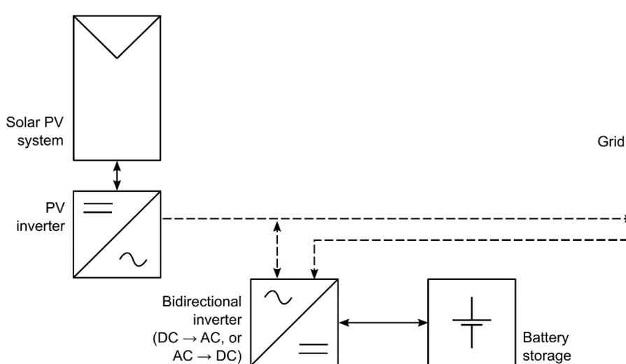
**Figure 16: Solar PV system with battery storage, AC-coupled to the grid, following [38]**
