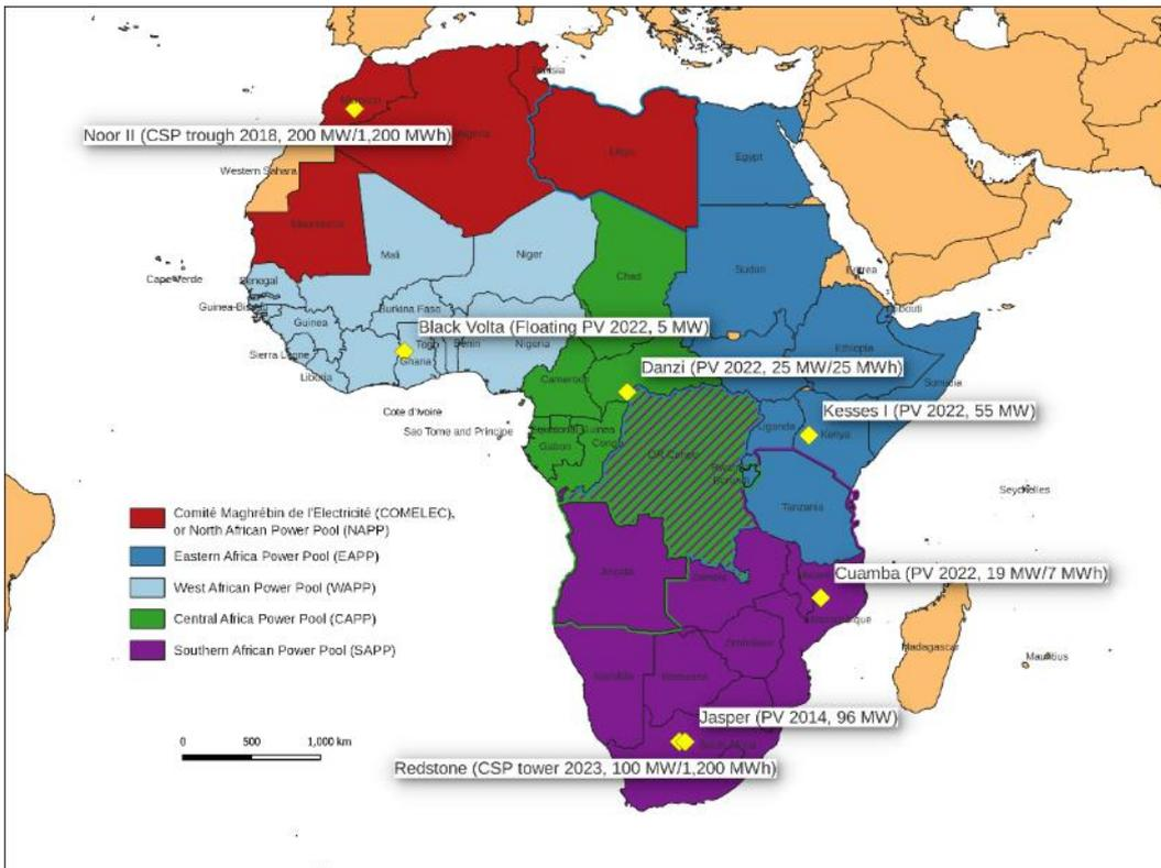
Figure 3: Cases detailed in this study, with their locations in the Power Pools, characterized by name, technology type, rated power and storage capacity (where applicable)
