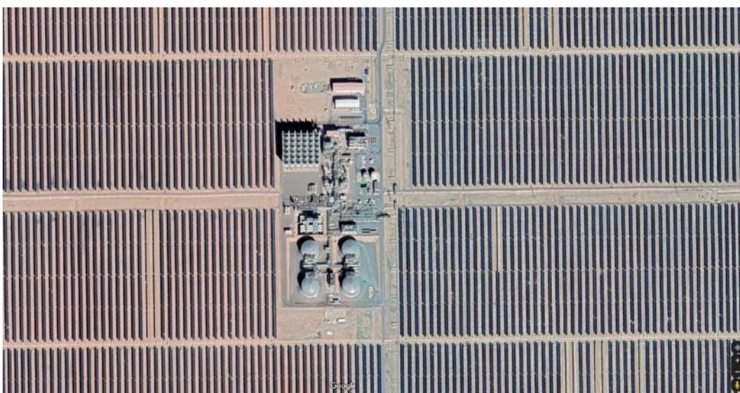
Figure 4: Aerial photograph of the Noor II power plant with mirror lines; in the centre the power block with air cooled condensers and hot/cold storage tanks is seen. Source: Google
