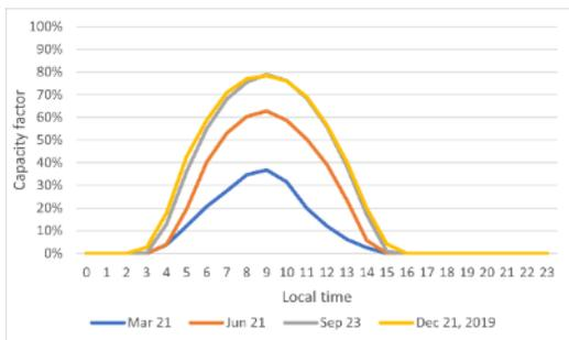
**Figure 41: Simulated capacity factors for PV power plant in Cuamba, Mozambique; hourly distribution during four days in 2019. Data source: [87]**
