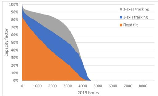
**Figure 53: Hourly capacity factors 2019 for the Jasper PV plant (fixed tilt installation), and hypothetical power plants with 1-axis and 2-axes tracking at the same location**
