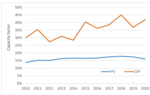
**Figure 54: Capacity factors of PV and CSP power plants installed worldwide. Source: [31]**
