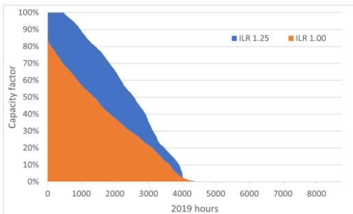
**Figure 50: Hourly capacity factors 2019 for two Inverter Loading Ratios (ILR), for the solar irradiance at Kesses I**
