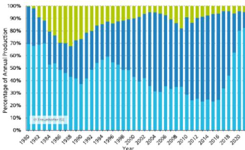
Figure 23: Breakdown of photovoltaic production according to cell technology. Source: [34]
