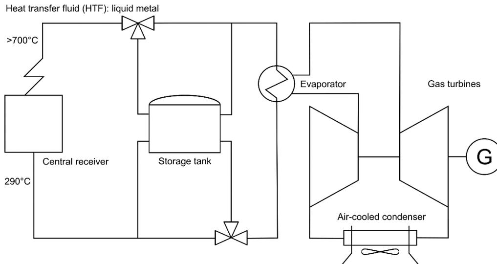
**Figure 19: Proposed layout of a future high efficiency Concentrated Solar Power (CSP) plant based on current solar tower central receiver technology. Improvements include high-temperature heat transfer fluids in receiver and storage loop. The power block runs a Brayton cycle. Following [37] [39]**
