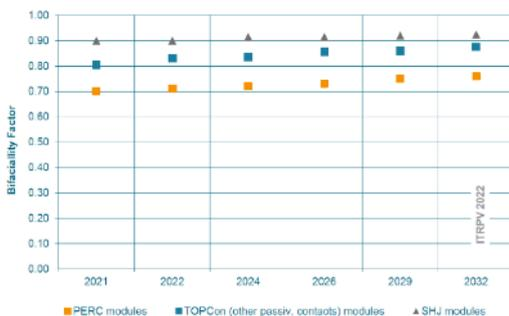
**Figure 26: Bifaciality factor of various PV technologies. Source: [74]**
