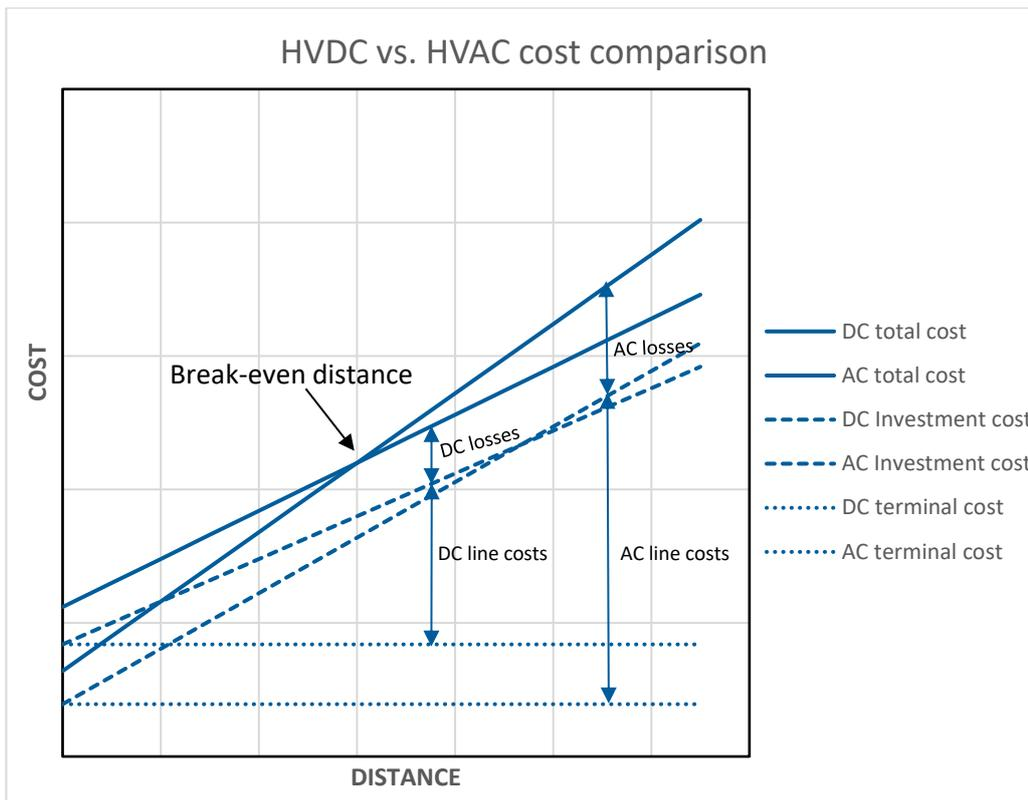
Figure 88. HVDC vs. HVAC costs [200]
