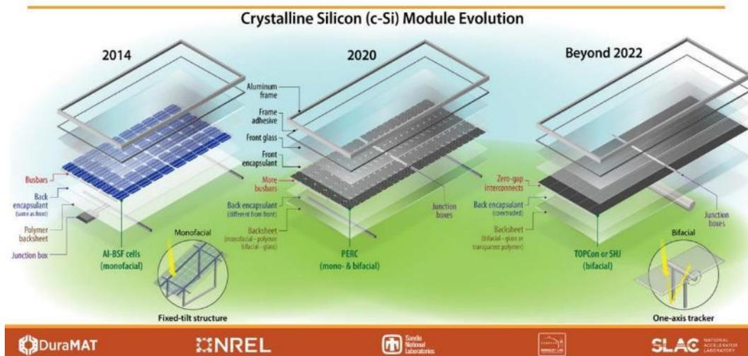
Figure 24: Photovoltaic crystalline silicon (c-Si) module trends. Source: [73]
