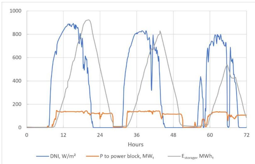
**Figure 18: Actual operational data of the 50-MW<sub>e</sub>-Concentrated Solar Power (CSP) plant *Andasol 2* (Spain) with parabolic trough collector field and 2-tank indirect storage configuration (see Figure 5) on June 26-28, 2010. Capacity of the molten-salt storage is 7.5 hours. The subscripts ‘t’ and ‘e’ refer to ‘thermal’ and ‘electric’, respectively. From [52]**
