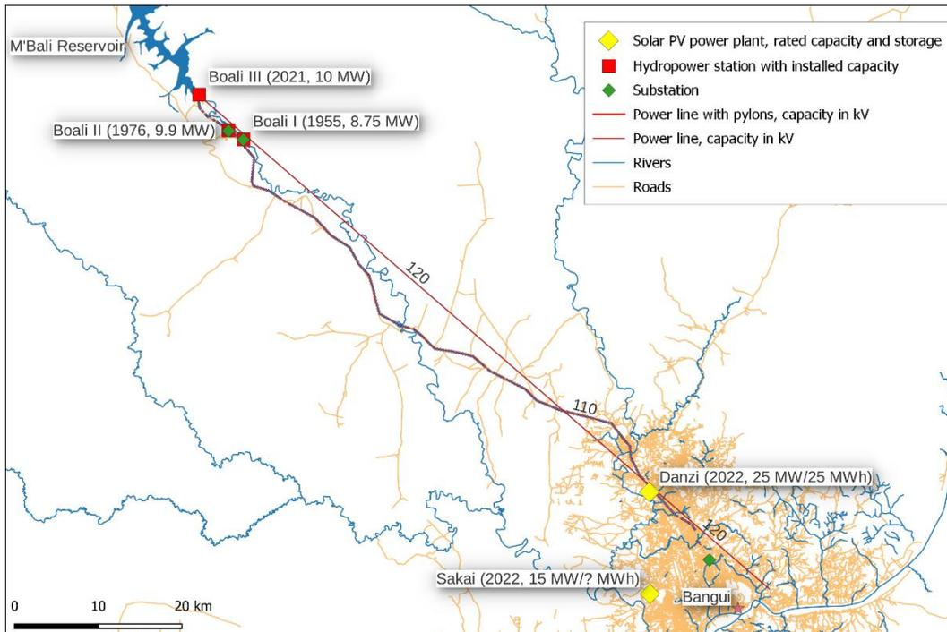
**Figure 10: Danzi PV power plant north-west of Bangui, capital of the Central African Republic. The Danzi PV power plant connects to an existing power line between the Boali I-III hydroelectric power stations and Bangui. The map illustrates two paths of the power line, an approximated straight line [19] and the actual path [20] along the RN 1 road**
