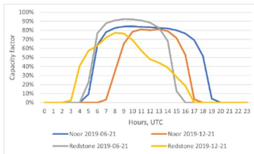
**Figure 47: Hourly capacity factors for the solstice days of 2019, for the CSP power plants' solar fields Noor II and Redstone. Source: [87]**
