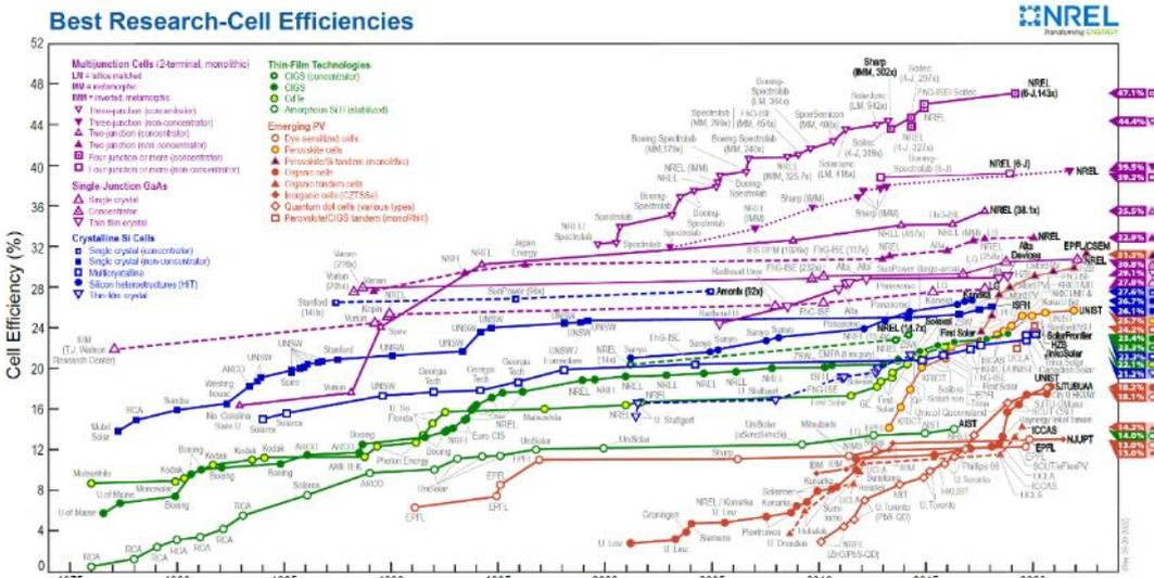
Figure 22: Best research-cell efficiencies. Sun-to-electricity efficiency of laboratory scale cells. Source: [72]
