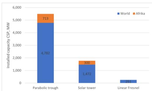
**Figure 12: Cumulative installed capacity of Concentrated Solar Power (CSP) plants in Africa and the World. Source [31]**
