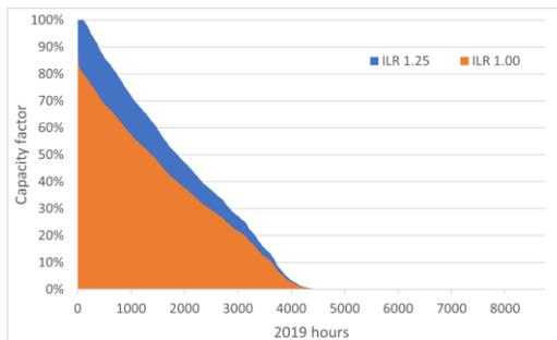
**Figure 51: Hourly capacity factors 2019 for two Inverter Loading Ratios (ILR), for the solar irradiance at Jasper**
