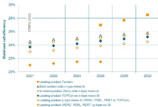
**Figure 25: Average stabilized efficiencies for Si solar cells in mass production. Source: [74]**
