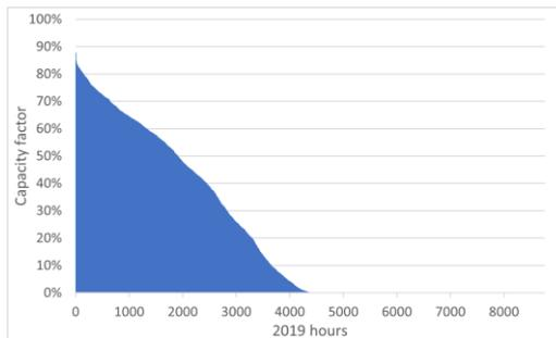
**Figure 40: Simulated capacity factors for PV power plant in Cuamba, Mozambique; hourly distribution histogram 2019. Data source: [87]**
