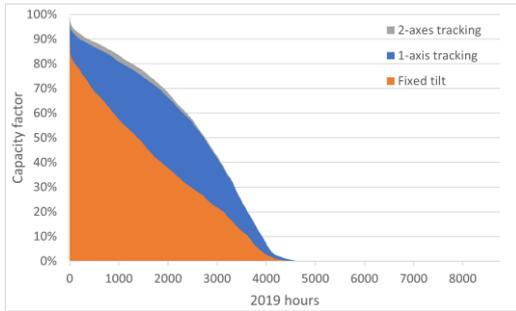
**Figure 52: Hourly capacity factors 2019 for the Kesses I PV plant (1-axis tracking installation), and hypothetical power plants with fixed tilt and 2-axes tracking at the same location**
