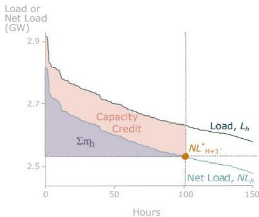
**Figure 55: Load and Net Load Duration Curves for Peak Hours (Top 100 peak hours) of the Year.**
