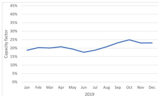
**Figure 42: Simulated capacity factors for PV power plant in Cuamba, Mozambique; monthly averages for 2019. Data source: [87]**
