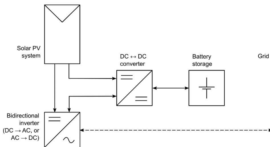
**Figure 15: Solar PV system with battery storage, DC-coupled to the grid, analogous [39] [38]**
