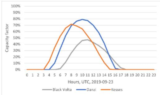
**Figure 44: Hourly capacity factors for 23 Sep 2019, simulated, for the PV plants Black Volta, Danzi, and Kesses I, UTC time. Source: [87]**
