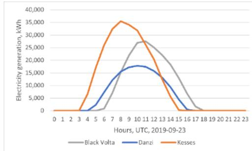
**Figure 45: Hourly energy generation for 23 Sep 2019, simulated for the PV plants Black Volta (65 MW), Danzi (25 MW), and Kesses I (55 MW), UTC time. Source: [87]**
