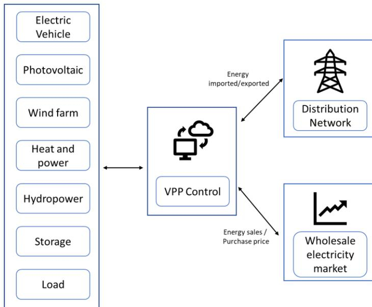
**Figure 90. Diagram of a VPP and interaction with electricity network and market [210]**
