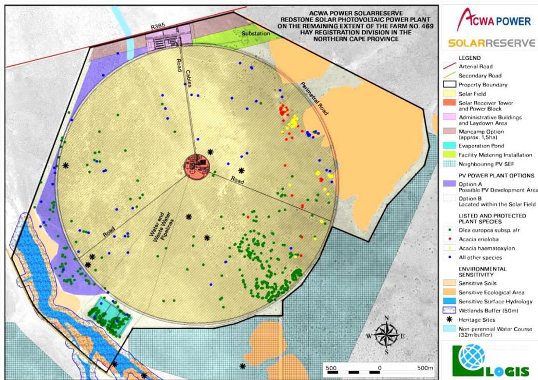
Figure 7: Environmental Management of the Redstone CSP plant: Sensitivity map of the power plant development footprint. Source: [14]
