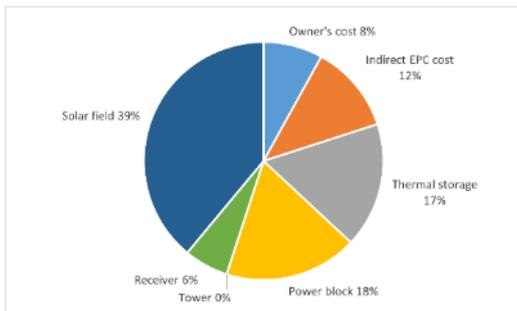
**Figure 58: Cost breakdown of a CSP plant based on parabolic trough technology. Source: [31]**
