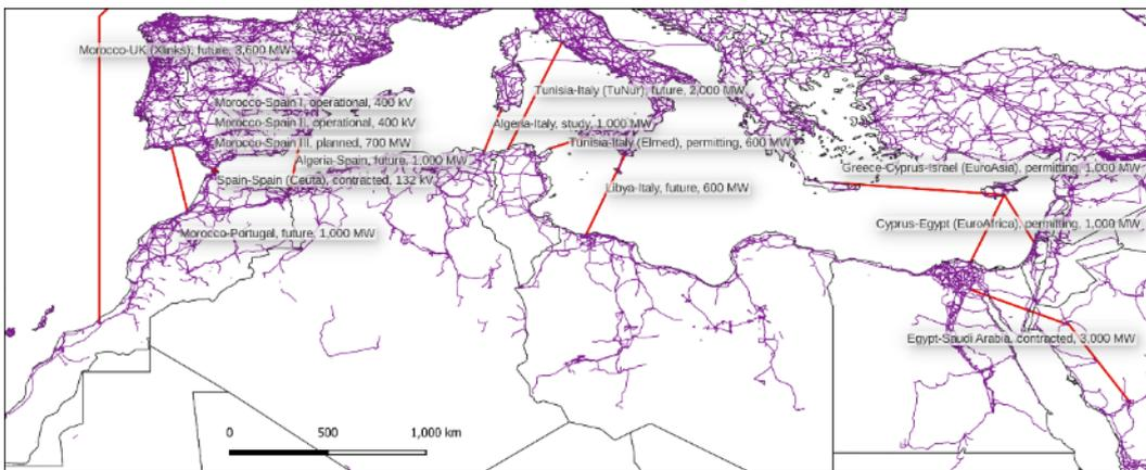
**Figure 83: Undersea cables between Africa and Europa, as well as between Africa and Arabia, with status, voltage, or power capacity where available. Sources: [139] [140] [141] [142], for details see Table 12**
