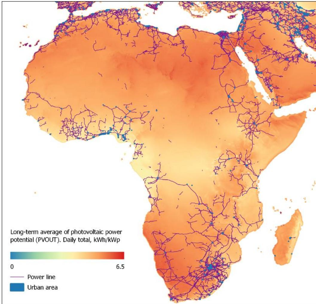
**Figure 81: The African transmission grid [20], urban areas, with a map of the long-term average of photovoltaic power potential (PVOUT) [3]; note the large areas without transmission grid, and the gaps between regional grids**
