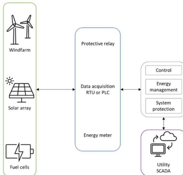
**Figure 92. SCADA systems for renewable energy management based hybrid power system [227]**
