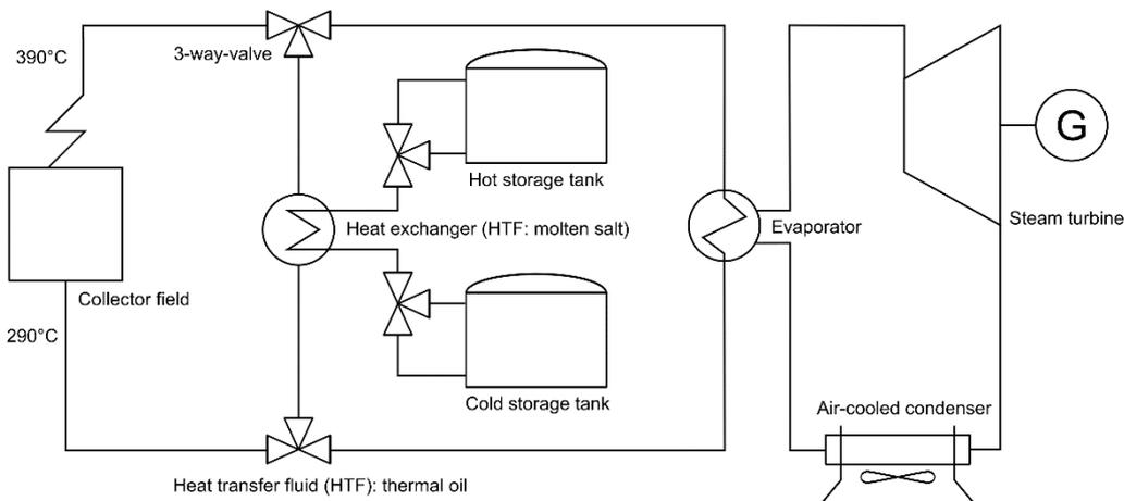
**Figure 5: Schematic of the Noor II CSP power cycle. Note the 2-tank indirect storage configuration. ‘Steam turbine’ is a simplification of the power block running a Rankine steam cycle. Sources: [8] [9]**
