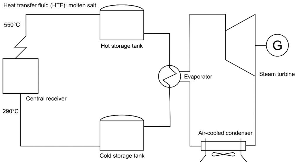
**Figure 6: Schematic of the Redstone CSP plant. The storage tanks are positioned directly in the molten salt loop. ‘Steam turbine’ is a simplification of the power block, running a Rankine steam cycle. Sources [10] [11] [9]**
